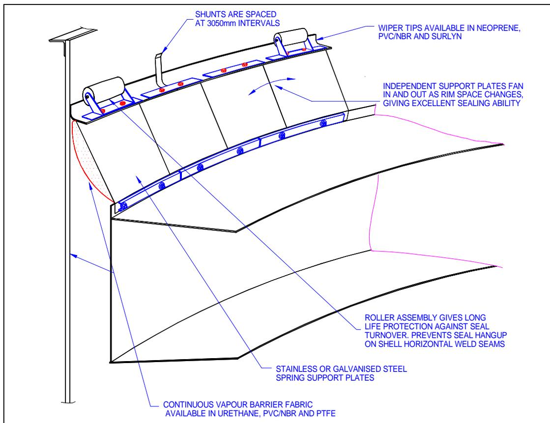
A significant feature of the seal is the special synthetic roller assembly. These positively eliminate seal roll over. Ideal for old out-of-round tanks. The corrosion free roller is shell-contoured to minimise painted shell marking. The roller assembly allows a shorter support plate height for a given maximum rim space. This allows greater working tank volume. The roller normally only contacts the shell when the rim space is larger than nominal.
